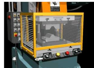
9.6 A fixed guard is a permanent machine part that completely encases potential hazards. Fixed guards provide maximum operator protection. Interlock guards are connected to a machine's power source. If the guard is opened or removed, the machine automatically disengages. Interlocking guards are often preferable
